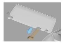
With the sun visor in its stowed position, slide the battery holder towards the front of the vehicle.
