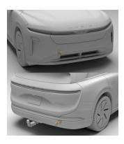
3. Attach the winch cable to the tow eye. The pull angles must not exceed 5 degrees from center either up or down and 25 degrees from center either left or right.
