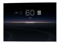
During regenerative braking, the charge/ power meter horizon line that sits below the speedometer shows the current amount of energy being generated and fed back to the high-voltage battery.
