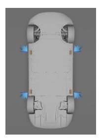
Ensure that any non-Lucid repair facility servicing your vehicle is aware of these lifting points when raising your vehicle on a lift.
