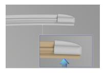
Check the blade rubber for cracks, splits, or roughness. Immediately replace the blade if any damage is found, to prevent damage to the glass.
