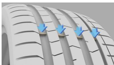
Tires fitted as original equipment have tread wear indicators molded into the tread pattern.
