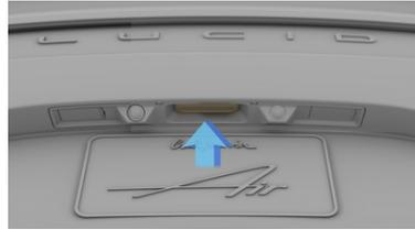
2. Open the trunk and remove the towing device from under the right-side trunk floor panel.
