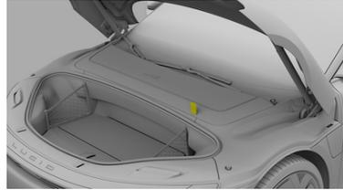
You can determine the location of the cut loop by the yellow label wrapped around it. This label should be visible, even with the maintenance access panel in place.
