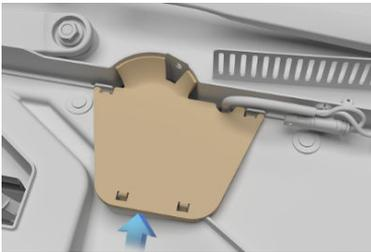
3. Check the fluid level visually by looking at the outside marks on the side of the reservoir without removing the filler cap.
