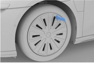
2. Starting with one spoke, pull on the outer edge of the spoke to release. Repeat for each spoke until all of them are released.
