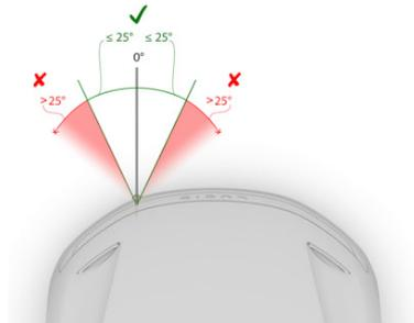
2. Position the towing device through the bumper and rotate it clockwise into the attachment point on the body until it is fully seated. The towing device shaft should be parallel to the ground.
