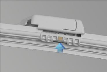
If a washer jet nozzle's performance may decrease if it becomes clogged with debris or build-up. There are several methods for removing any blockage:
