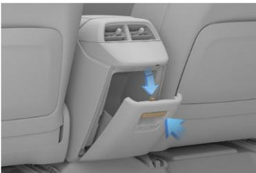
Pull the latch to release the storage compartment cover and allow it to open. Press the cover to close.
