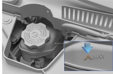
The brake fluid level should always be between the **MIN** and the **MAX** marks.
