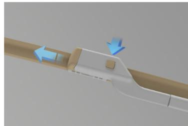
4. Installing a new wiper blade involves the reverse procedure of removing it. You should be able to hear and feel it click into place on the wiper arm.
