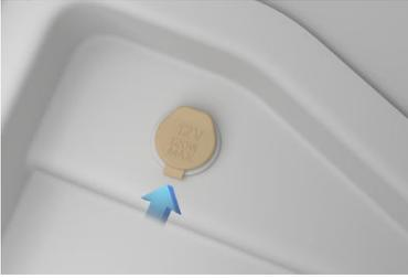
The power socket is primarily provided for use with the tire repair kit, but can also be used for other accessories requiring up to 15A or a maximum of 180 watts.
