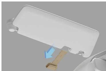
With the sun visor in its stowed position, slide the battery holder towards the front of the vehicle.
