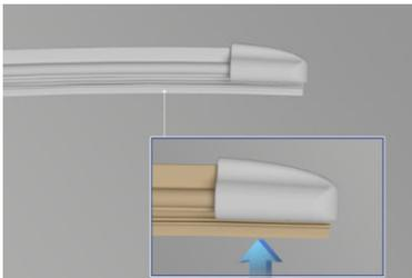
You should periodically check and clean the wiping edge of the wiper blade. Clean the blade edge using a soft cloth or sponge, and isopropyl (rubbing) alcohol or windshield washer fluid. Also, check the blade rubber for cracks, splits, or roughness. Immediately replace the blade if any damage is found, to prevent damage to the glass.
